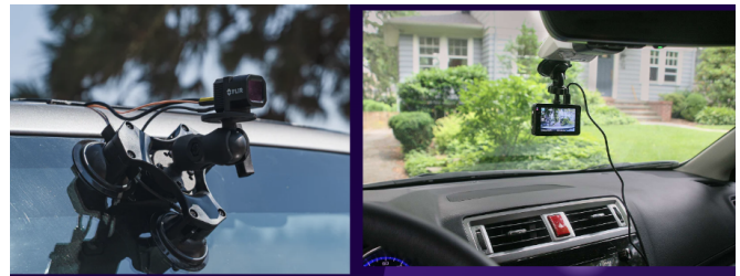
Figure 1: Thermal and dash camera set-up on the vehicle.
