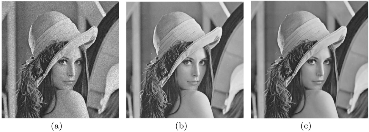
Fig. 11. (a) Lena image corrupted by the Rayleigh noise with \sigma_\eta = 5 , (b) denoised image obtained using BM3D method, RMSE=0.0051, and (c) denoised image obtained using the proposed method, RMSE=0.0023.
