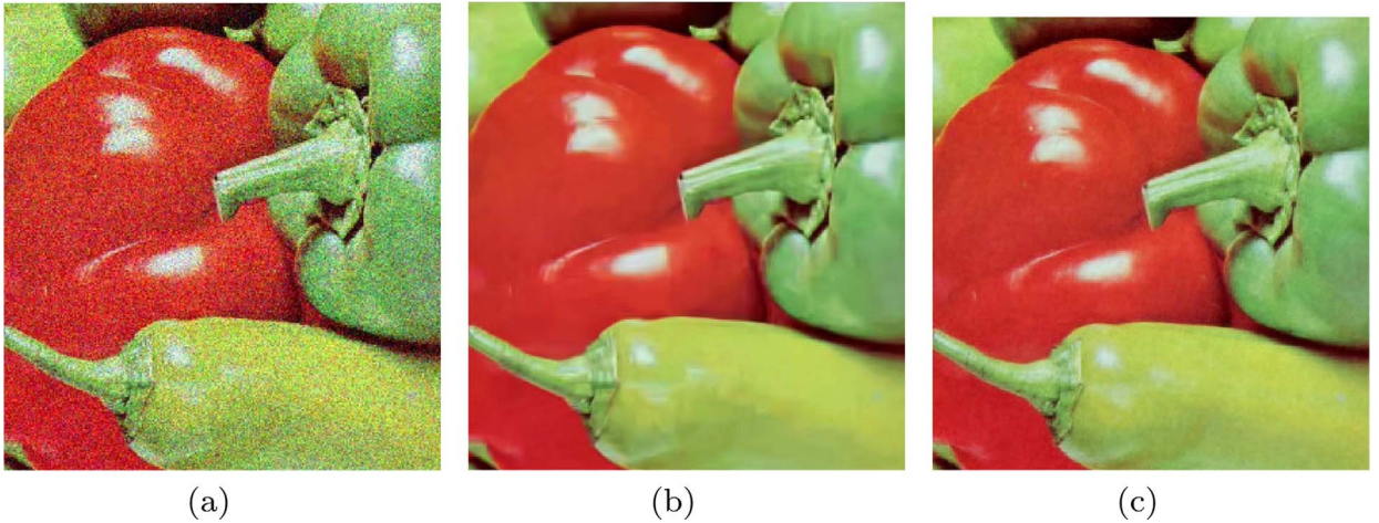
Fig. 16. Color image denoising; (a) cropped noisy Peppers image with \sigma_\eta = 30 , PSNR=18.59 dB as well as the corresponding denoised images obtained using (b) CBM3D, PSNR=30.61 dB and (c) the proposed CT-Tri-SaS-MMAE, PSNR=30.42 dB.
