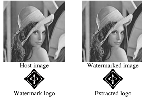
Figure 2 . The host image, its watermarked, watermark and extracted logo; PSNR=74.17 , NC=1 and a=0.5.
